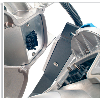
Built-in safety knife connector system, which automatically disconnects the mains power when the rear-access back cover is opened
