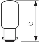
Energy consumption kWh/1000h 20 kWh • Measuring Conditions 4000X Switching cycle • Product Dimensions Overall Length C 52 (max) mm Diameter D 22 (max) mm • Product Data 924132044240 Order code 924132044240 Full product code Full product name CL SM 1CT Order product name SM 1CT Pieces per pack 1 10X10F Packing configuration Packs per outerbox 100 Bar code on pack -8711500250230 EAN1 8711500251329 Bar code on intermediate packing -
