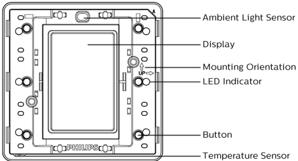
The AntumbraDisplay Panel application module consists of six buttons, LED indicators, a temperature sensor, an ambient light sensor and a proximity sensor.
