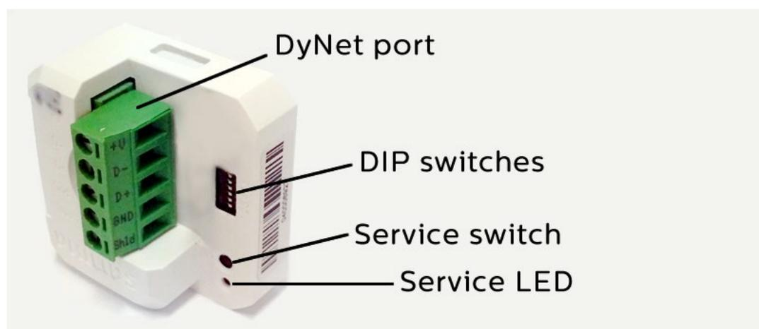
The DyNet communication module is common across the Antumbra series. It contains all the logical and network functions required by the panel.
