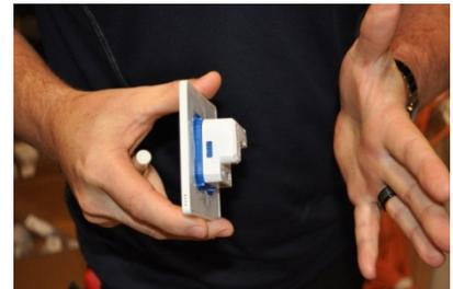
To separate the communication module and application module, use a small screw driver to gently unlock the two clips on either side of the communication module.
