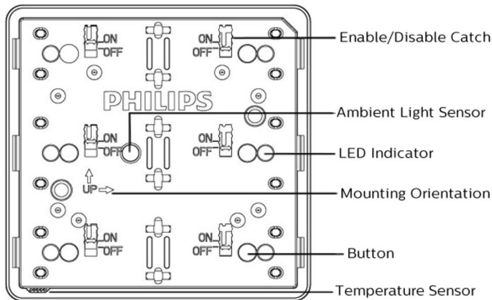
The AntumbraButton Panel application module consists of six configurable buttons, indicator and backlight LEDs, a temperature sensor, an ambient light sensor and a proximity sensor.
