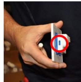
The mounting plate fits any standard size European wall box or a wall cutout of 51x 51 mm. If using wall mounting then the smaller base mounting screw locations should also have a small indent behind them, made into the wall so there is no interference from the screws while mounting the panel. The Mounting box must have a depth of at least 33 mm to contain all the panel components and network cabling. Remember that the wall box needs space for two cables.
