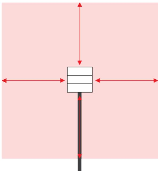
The first 30cm of the cable should be fixed and if possible bent and exiting towards the bottom of the panel as shown above
