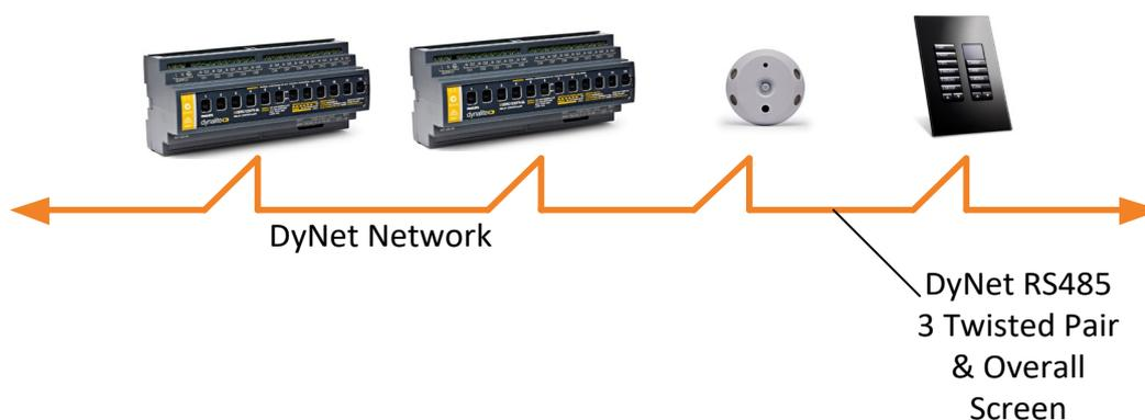
Unplug the five way screw socket on the back of the Communication module. Terminate the network cable following the diagram below. All devices must be terminated correctly as shown.
