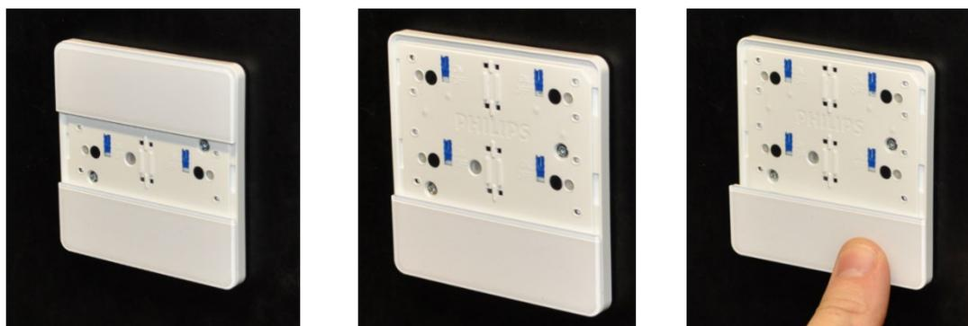
After ensuring that the correct buttons are enabled or disabled as required, attach the buttons to the application module. Carefully line up each button with the application module, then press the center of the button until it clicks into place. Press each side of the button into place.
