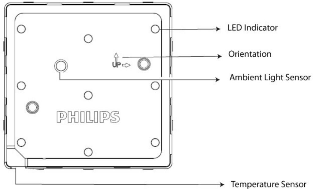
The AntumbraTouch Application Module has six configurable touch points, LED indicators, a temperature sensor, a daylight sensor and a proximity sensor.
