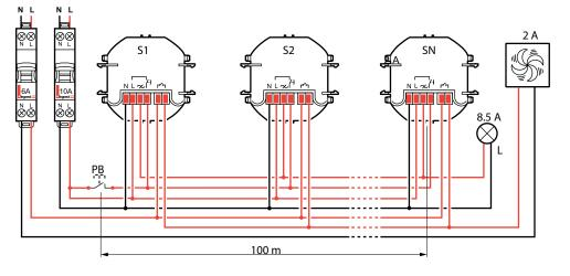
4.3 Wiring for several loads connected in parallel
