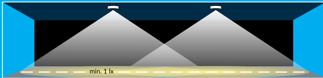
ESCAPE ROUTE LIGHTING | OPTIMAL FOR ESCAPE ROUTES WITH A HEIGHT ABOVE 7 M
